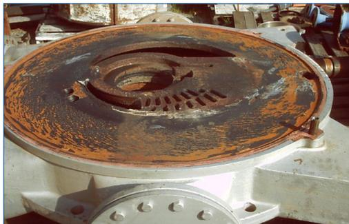
Erosion-corrosion damage on port plate
