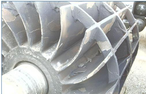
Damaged rotor before rebuilding
