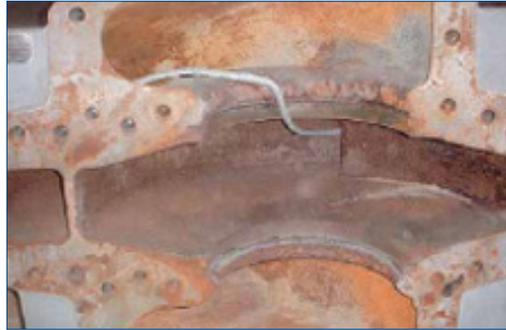
Corroded and cavitated pump
